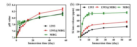
Fig. S2 (a) pH value changes of the immersion medium; (b) Concentration of Si ion released from the scaffold into the medium as immersed in SBF; mean  $\pm$  SD, n = 5.
