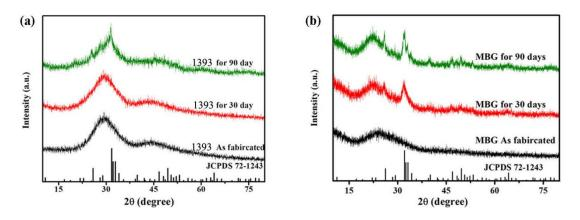
Fig. S1 XRD patterns for 1393 (a) and MBG (b) glass powder as immersed in SBF for 0 and 90 days. A reference hydroxyapatite (JCPDS 72-1243) is shown for comparison.
